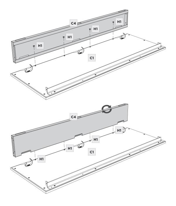
Connect (C2) Left Leg Frame to (C4) Wire Trough using 2 (H1) Screws. Fasten to (C1) Top Panel Connection Tab using 1 (H1) Screw. Partially tighten screws.
